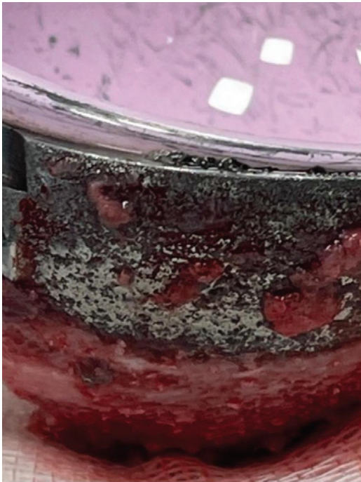
FIGURE 5 | Metal residues from fracturing corrosion, predominantly titanium.
